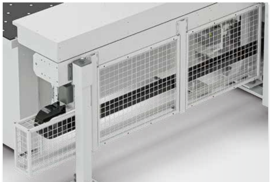
The lower safety fence prevents entry into the working area.
