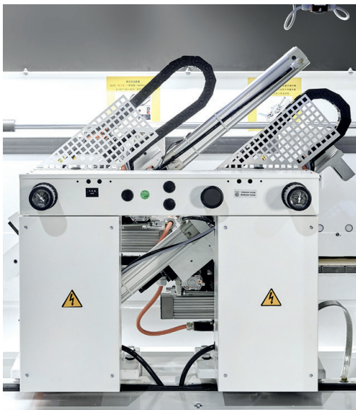
Snipping unit: With exact cuts the face side can be snipped either straight or with chamfer.
