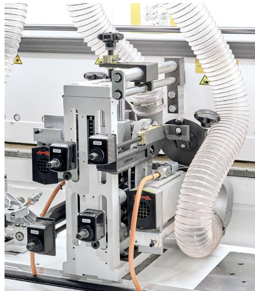
Chamfer/radius trimming unit: This 2-point adjustment trimming unit is ideal for rapid changes between thin and thick edges.
