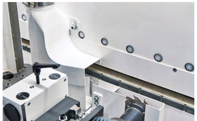
Grooving unit: effective suction hood
