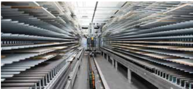
Collating between format and edge banding and drilling: Buffering and collating e.g. for assembly and tour order or color, form, dimensions etc..
