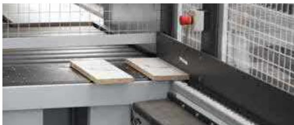
Manual parts supply: At the manual workstation, workpieces are passed on to the collating center manually. The workpieces are stored temporarily and sorted in the SORTEQ before being forwarded to the next production step.
