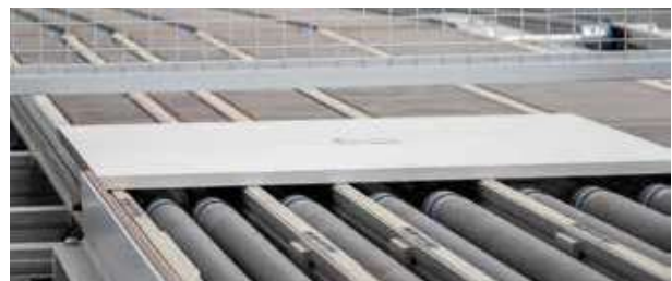
Material transfer from the SORTEQ R-200: Workpieces are forwarded on to the subsequent processing step on an order-by-order basis via transport routes that are connected to the collating center.
