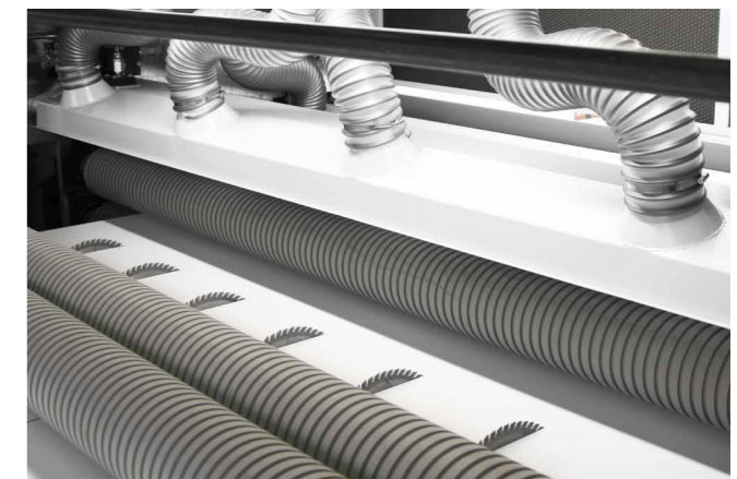
Ground transport rollers
