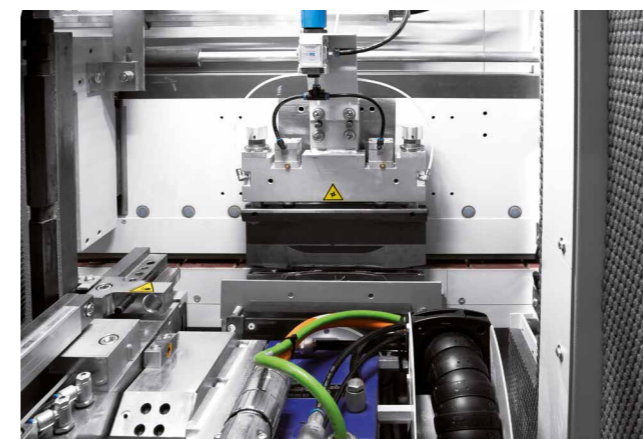
Pressure and support pad for laminate flooring to protect the chain and ensure precision processing. Additional support is provided for the workpiece in the area of the processing unit.
