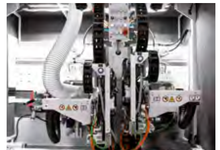
High-power trimming unit SF30 with automatic adjustments
