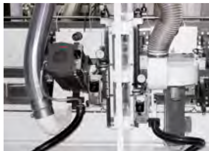
Unit guidance systems with high-precision setting device and swivel-mounted high-frequency motors
