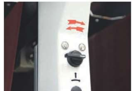
Optional Cutting direction • Cutting direction either with or against the feed direction. Different cut directions ensure maximum fiber reduction. Particularly important when combined with water-based paint systems
